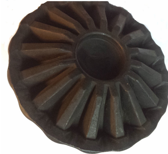
Fig. 2 – Precision forged bevel gear with straight teeth (Turcilă, 2015b).
